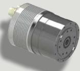
gear has a minimal backlash. The integrated output bearing can withstand high radial and axial loads and also withstands tilting torques. You can utilize all the advantages of the gear motor in combination with our RoboDrive technology, e.g. higher dynamics due to a stiffer powertrain. Combinations of RoboDrive motors and Eppinger gears can be tailored to customer requirements.
